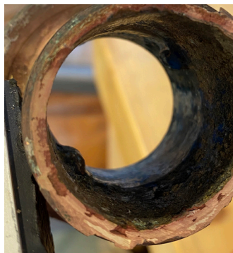
Fig 2 Note the coppery flecks through the body
